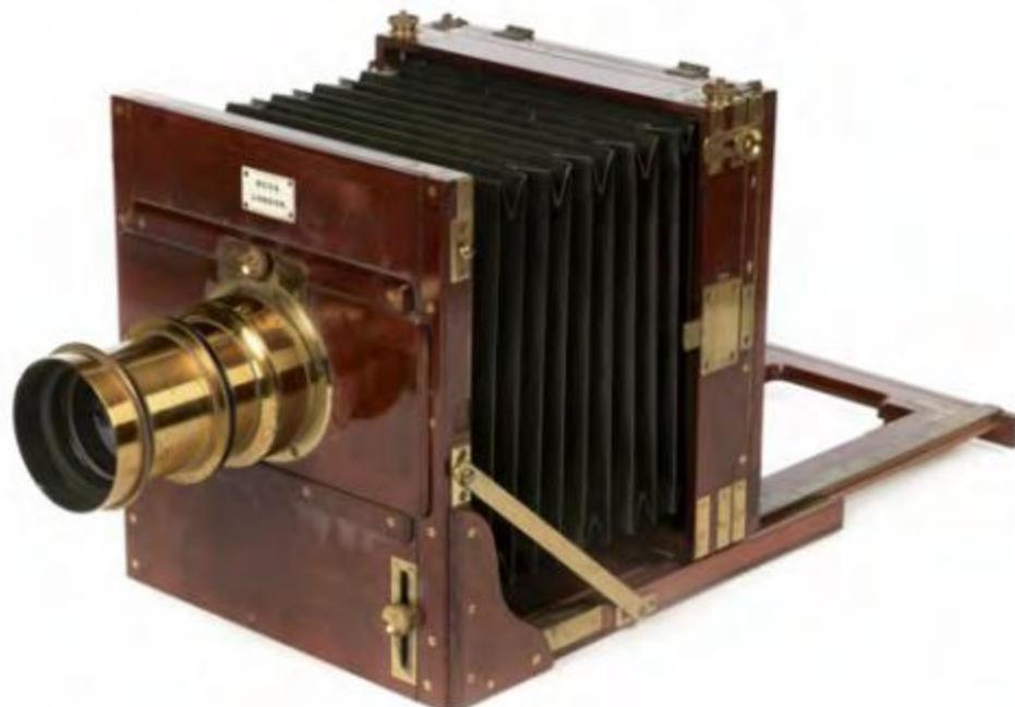
112\* **Ross of London.** Ross of London mahogany and brass 6 1/2 x 8 1/2 full plate camera with substantial brass lens marked "E. Suter, Basle, No 4680, Aplanat B No 6, 16x13", centre ring on lens barrel adjusts aperture, black square bellows which appear to be in good condition, vertical and horizontal sliding movement of the front standard, rack and pinion focusing, complete with mahogany plate holder and leather carry case (worn and some damage)
